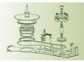
A Spider rebuild should be completed every six months to a year, depending on usage and wear in production.
