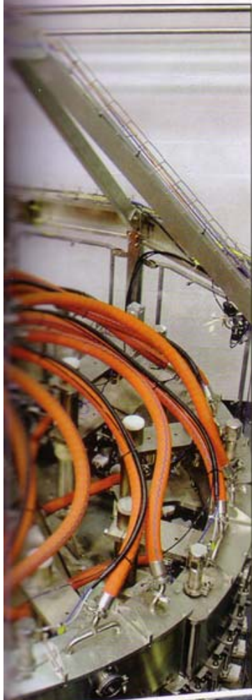
Each GlobalFill machine (left) features ten filling bowls with six heads and benefits from the UK-designed Mayhew valve
